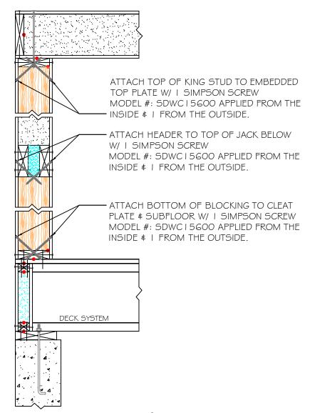
NOTE: ALL RED DOTS - APPLY CONTINUOUS 3/8" DIA. BEAD OF MASTIC SEALANT AT WOOD TO FOAM \$ WOOD TO WOOD CONNECTIONS AT INTERIOR SIDE.
