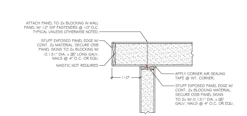
NOTE: ALL RED DOTS - APPLY CONTINUOUS 3/8" DIA. BEAD OF MASTIC SEALANT AT WOOD TO FOAM \$ WOOD TO WOOD CONNECTIONS AT INTERIOR SIDE.
