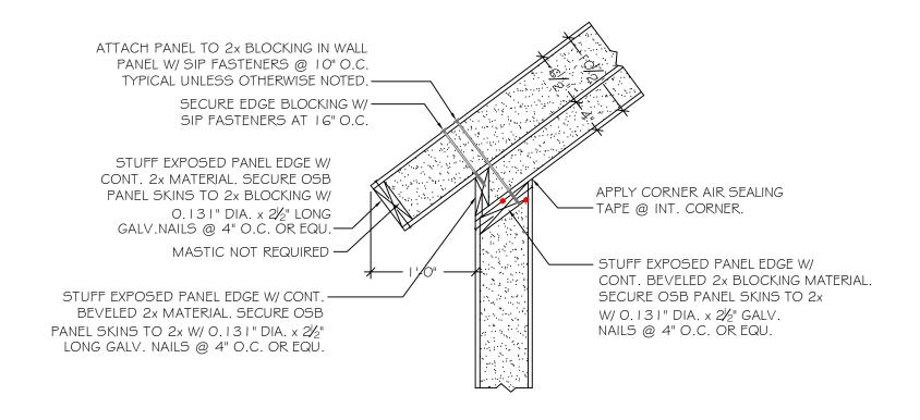
NOTE: ALL RED DOTS - APPLY CONTINUOUS 3/8" DIA. BEAD OF MASTIC SEALANT AT WOOD TO FOAM \$ WOOD TO WOOD CONNECTIONS AT INTERIOR SIDE.
