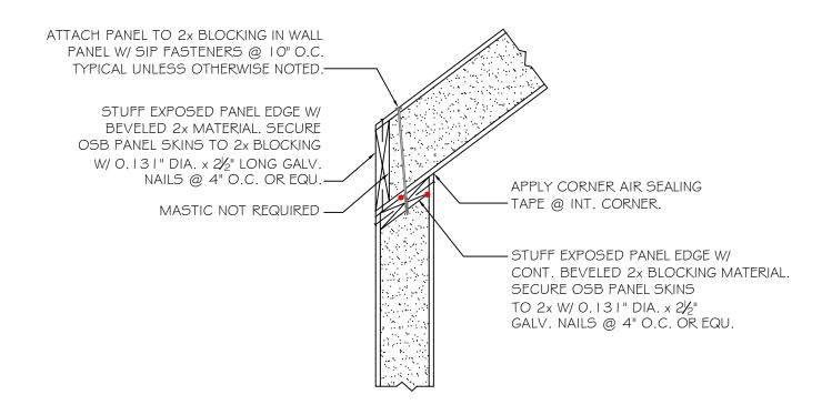
NOTE: ALL RED DOTS - APPLY CONTINUOUS  $\frac{3}{8}$ " DIA. BEAD OF MASTIC SEALANT AT WOOD TO FOAM \$ WOOD TO WOOD CONNECTIONS AT INTERIOR SIDE.
