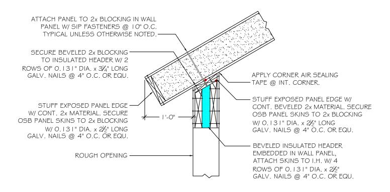
NOTE: ALL RED DOTS - APPLY CONTINUOUS 3/8" DIA. BEAD OF MASTIC SEALANT AT WOOD TO FOAM \$ WOOD TO WOOD CONNECTIONS AT INTERIOR SIDE.
