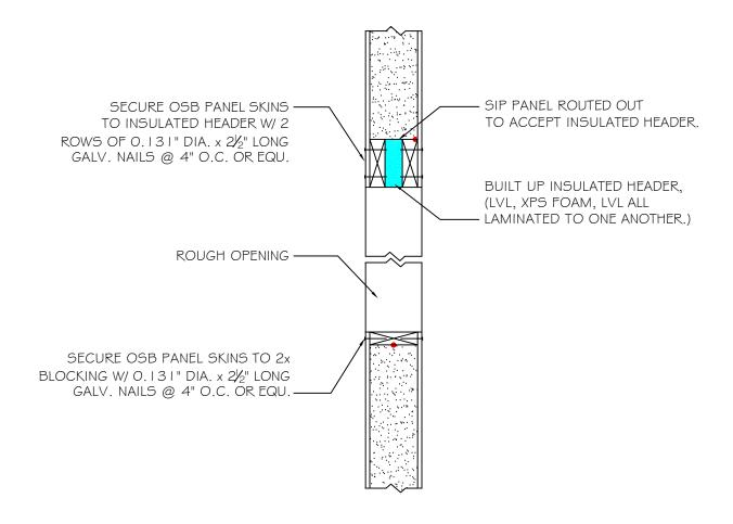
NOTE: ALL RED DOTS - APPLY CONTINUOUS 3/8" DIA. BEAD OF MASTIC SEALANT AT WOOD TO FOAM \$ WOOD TO WOOD CONNECTIONS AT INTERIOR SIDE.
