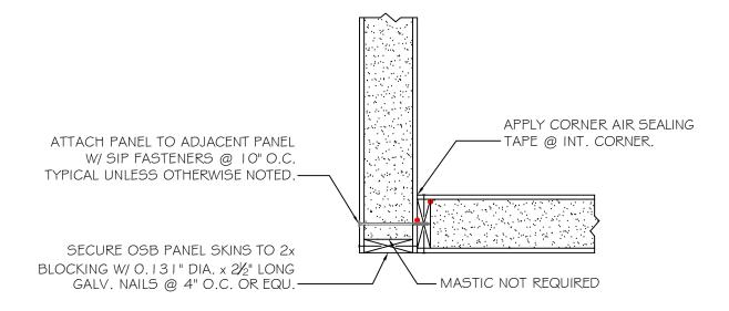
NOTE: ALL RED DOTS - APPLY CONTINUOUS  $\frac{3}{8}$ " DIA. BEAD OF MASTIC SEALANT AT WOOD TO FOAM \$ WOOD TO WOOD CONNECTIONS AT INTERIOR SIDE.
