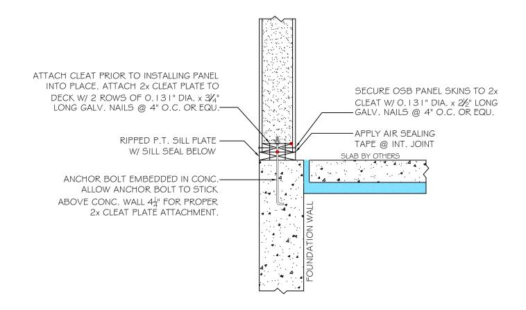
NOTE: ALL RED DOTS - APPLY CONTINUOUS 3/8" DIA. BEAD OF MASTIC SEALANT AT WOOD TO FOAM \$ WOOD TO WOOD CONNECTIONS AT INTERIOR SIDE.
