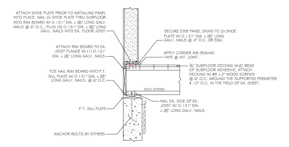
NOTE: ALL RED DOTS - APPLY CONTINUOUS 3/8" DIA. BEAD OF MASTIC SEALANT AT WOOD TO FOAM \$ WOOD TO WOOD CONNECTIONS AT INTERIOR SIDE.
