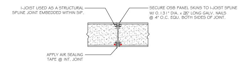
NOTE: ALL RED DOTS - APPLY CONTINUOUS  $\frac{3}{8}$ " DIA. BEAD OF MASTIC SEALANT AT WOOD TO FOAM \$ WOOD TO WOOD CONNECTIONS AT INTERIOR SIDE.
