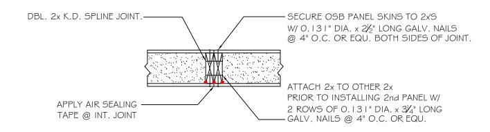
NOTE: ALL RED DOTS - APPLY CONTINUOUS 3/8" DIA. BEAD OF MASTIC SEALANT AT WOOD TO FOAM \$ WOOD TO WOOD CONNECTIONS AT INTERIOR SIDE.
