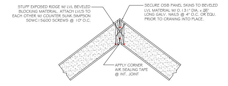
NOTE: ALL RED DOTS - APPLY CONTINUOUS  $\frac{3}{8}$ " DIA. BEAD OF MASTIC SEALANT AT WOOD TO FOAM \$ WOOD TO WOOD CONNECTIONS AT INTERIOR SIDE.
