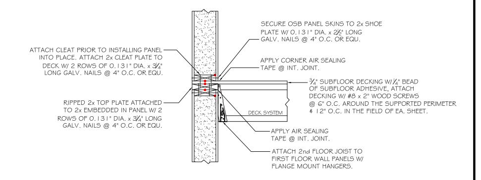
NOTE: ALL RED DOTS - APPLY CONTINUOUS 3/8" DIA. BEAD OF MASTIC SEALANT AT WOOD TO FOAM \$ WOOD TO WOOD CONNECTIONS AT INTERIOR SIDE.
