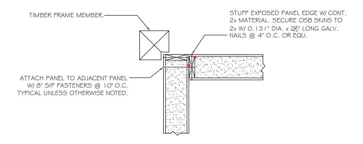
NOTE: PANEL BLOCKING INSTALLED ON THE GROUND PRIOR TO CRANING INTO PLACE TO ENSURE INTERIOR OSB SKINS GET FASTENED TO STRUCTURAL MEMBER EMBEDDED IN PANEL.
