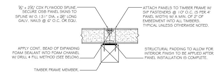
NOTE: IF PANEL IS ALREADY ROUTED FOR DBL. SPLINE CONDITION THAN INTERIOR SPLINE CHANNEL MAY BE USED AS WIRECHASE OR THE GAP SHOULD SIMPLY BE FILLED WITH EXPANDING FOAM SELANT.
