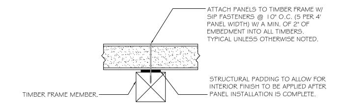
DETAILS ARE TYPICAL OF STANDARD CONDITIONS AND MAY NOT APPLY TO ALL PROJECTS. REFER TO FINAL PROJECT APPROVAL DRAWINGS FOR SPECIFICATIONS. PLEASE CONTACT FPI TECHNICAL DEPARTMENT FOR QUESTIONS AND/OR CONCERNS. PANEL TYPE: STRUCTURAL PANELS APPLIED DIRECTLY TO PADDED FRAME
